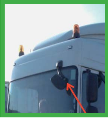
Pedestrian Safety Mirror a CRH requirement.
