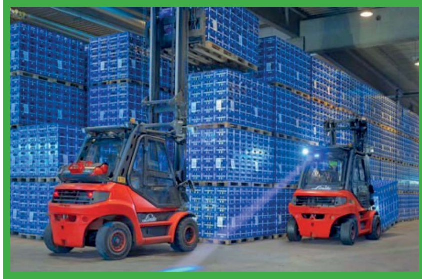
Blue Spot System in operation.
