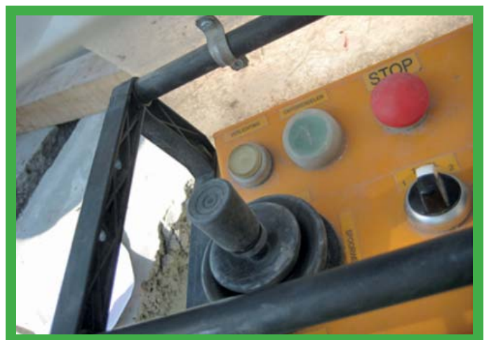
Dead Mans Joystick. You must push down to activate the joystick.
