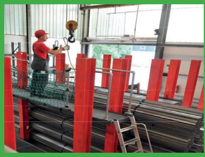
Safe access for attaching lifting hooks.
