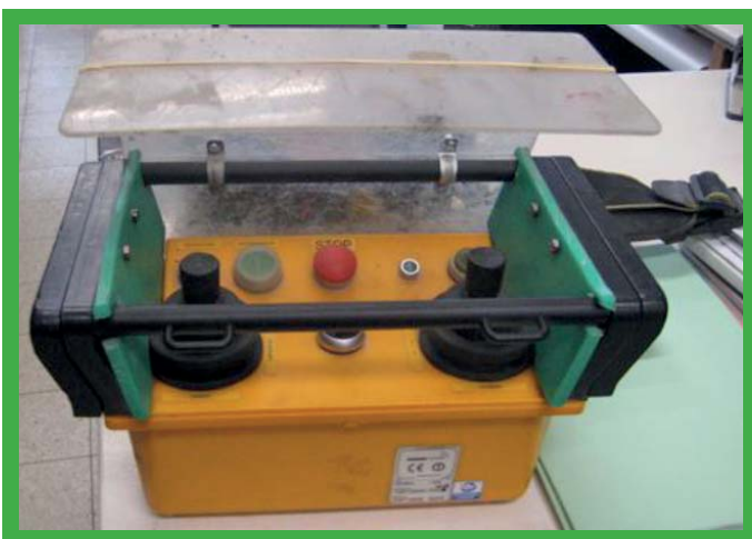
Dead Mans Joystick. You must push down to activate the joystick.
